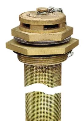
Of brass, 2"-thread, with flame arrester made from brass, 140 mm long, removable head, automatic pressure compensation, automatic vacuum compensation for curved surface (belly) of drum
