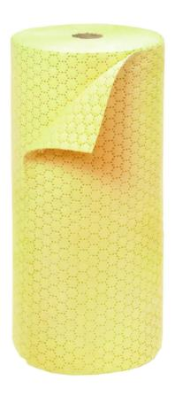
non-woven fabric binders made from polypropylene micro fibres in dispenser box with handles, dimensions: approx. 800 mm x 40 m lenghtwise transverse perforation, every 500 mm maximum absorption capacity per VE 162 l We recommend to use the smooth surface which is sublimated with spin fleece as working document.
